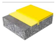
1. Scratch coat: Sikafloor®-21 PurCem® 2. Wear coat: Sikafloor®-21 PurCem®
