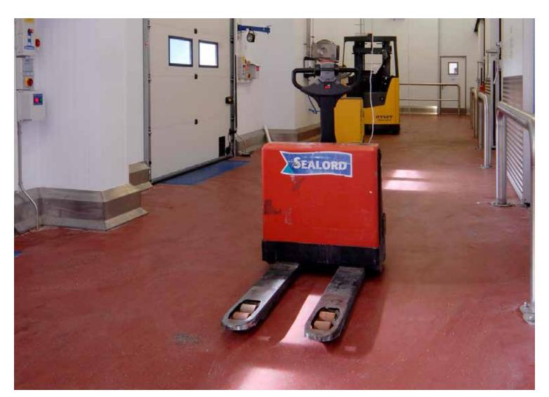
Pallet stackers and forklifts with small nylon or hard plastic wheels have high pointloads and cause extreme wear in frequently trafficked storage areas. Sikafloor® PurCem® HS-21 is a long life solution and hygienic choice in such conditions.
