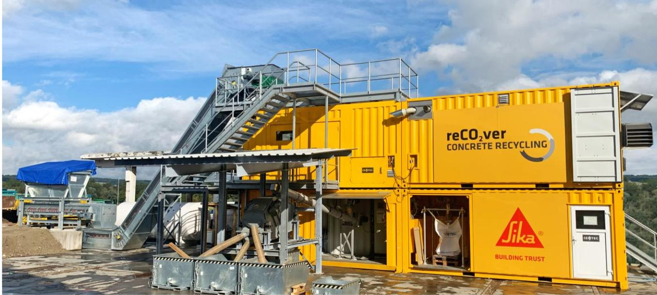
**Sika's recycling process for old concrete segregates concrete in its original ingredients to be re-used for new high-grade concrete**
