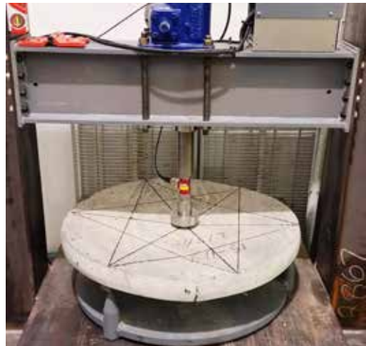
Figure 8.2.2.1: Standard Test Method for Flexural Toughness of FRC
