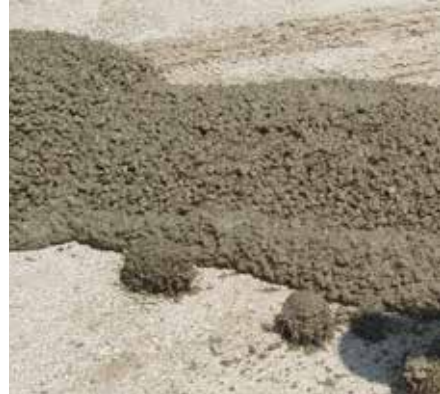
Figure 4.1.2: Fresh concrete with balling
