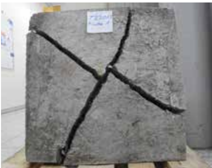
Figure 8.2.1.2: Underside view of tested square panels
