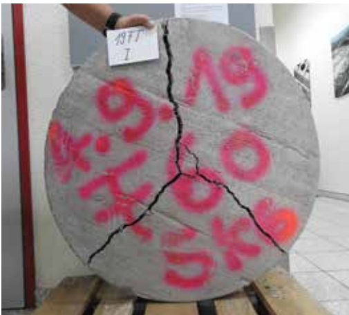
Figure 8.2.2.3: Specimen set up result reporting according to ASTM C-1550 round panel test
