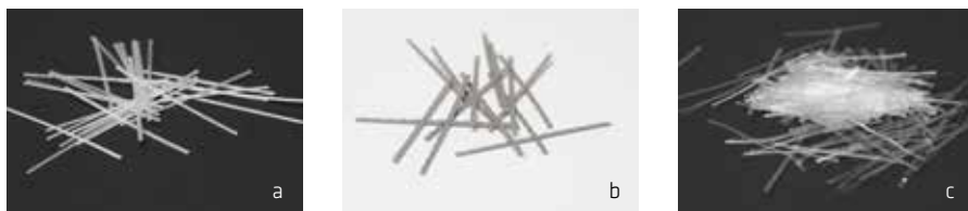
Figure 5.3.1: a) Straight embossed fibres b) Undulated fibres c) Soft flat fibres
