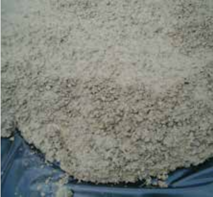
Figure 4.1.1: Fresh concrete without balling
