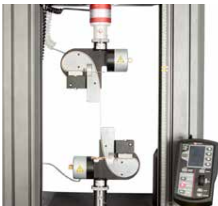
Figure 4.4.1.2: Snubbing clamp referred to ASTM D 2256-02
