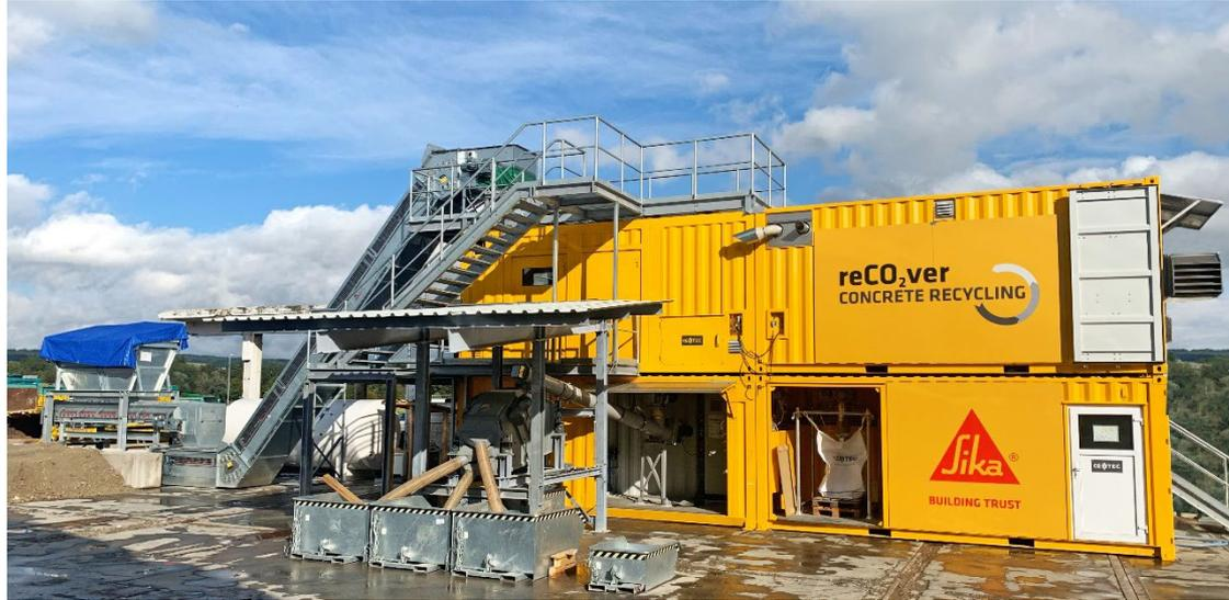
The reCO<sub>2</sub>ver<sup>®</sup> process separates old concrete into its component parts and uses regained material to produce new, high-quality concrete.
