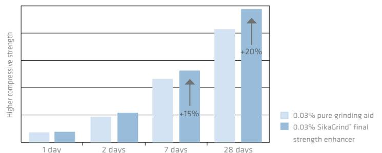
Early strength enhancement with SikaGrind® at increased production
