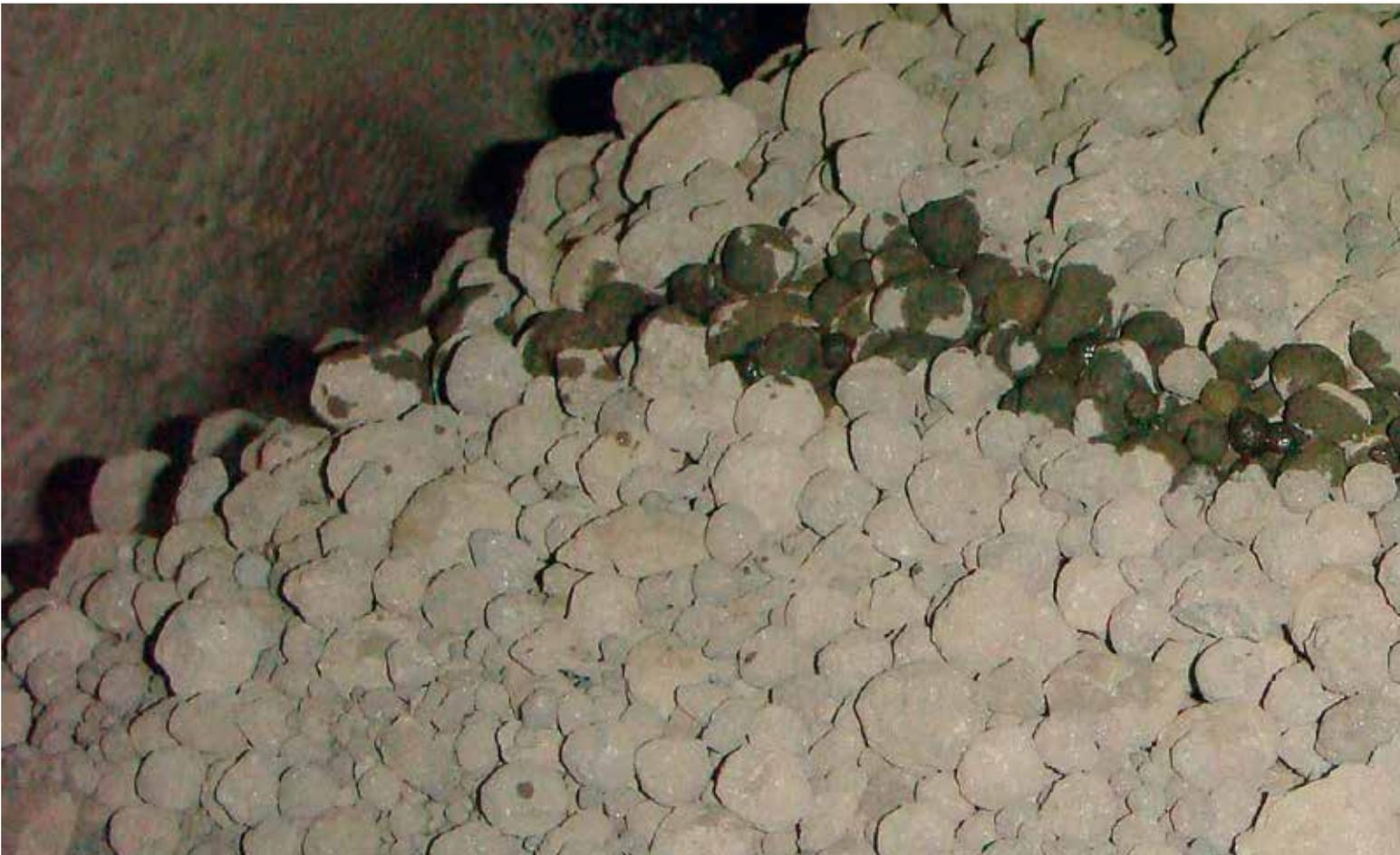
Grinding aids are added at low dosages, typically in a range of 0.02% - 0.05%, either onto the mill feed or directly into the mill itself. They reduce or even neutralise the surface energy by shielding the polarity to different degrees. As a consequence, the particles do not attract each other any more. Different effects can be observed:
