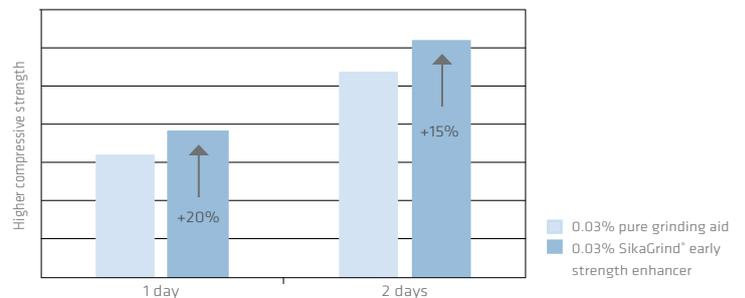
Strength enhancement with SikaGrind® due to increased fineness at constant production
