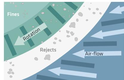
■ SikaGrind® ensures that the particles stay separated, thus enabling sufficiently fine particles to leave the mill and creating space for coarse particles to be refined.
