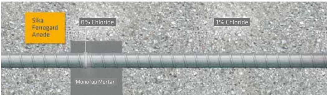
The Sika® FerroGard® Patch anode simply replaces the original corrosion anode, ensuring that the steel reinforcement in the vicinity of the repair remains cathodic – and protected from corrosion.
