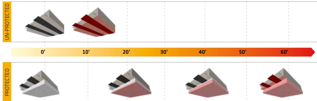
Even in the case of using protective materials applied in a considerable thickness, the expected protection will be restricted to a limited period of time
