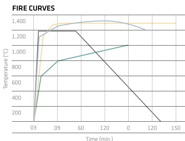
These fire exposure rating curves all simulate the temperature profile of a tunnel fire. The example of the Dutch RWS curve defines the maximum exposure which can be expected in the worst case scenario: This is defined as a fire of a road tanker truck with a load capacity of 50 m<sup>3</sup> that is 90% full of liquid hydrocarbon fuel (petrol).
