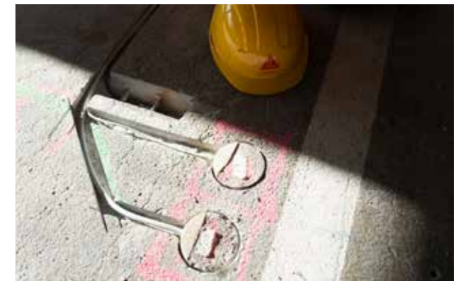
DuraMon multisensory were installed in well defined locations in the existing concrete structures. Some of these locations were protected with Sikagard® or Sikafloor® coatings, while the rest remain untreated (reference areas). The following photos show the installation on the construction site.
