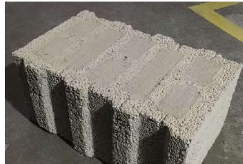
Example of a filled concrete block with insulating foam
