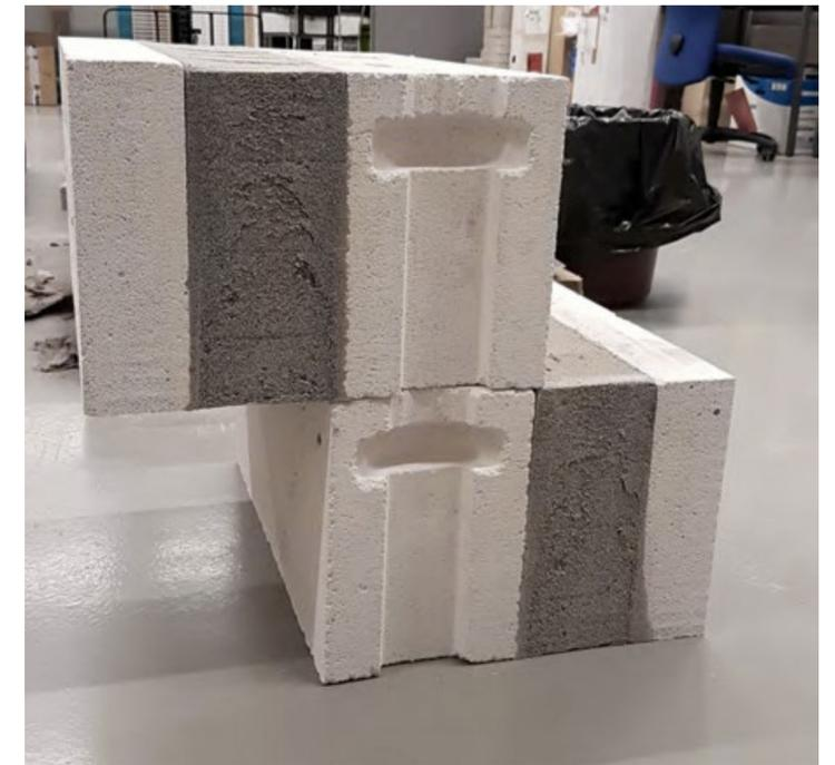
Example of insulated double-layer masonry. MasterProtect NFF 2000 IN insulates the wall and holds the facing formwork without reinforcement.
