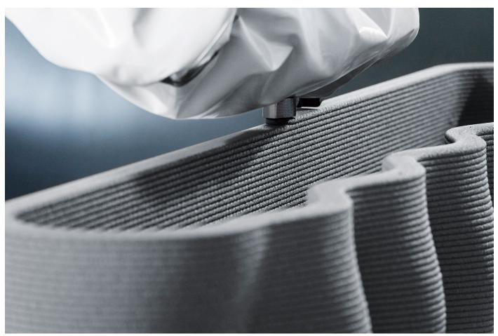
Sika's 3D concrete printing technology allows complex geometries to be realized economically.
