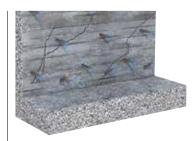
**3.** Fix the button head (non-return) fittings on the first packer and start the injection process at the lowest row of drill holes.
