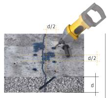
Drill holes for the packer alternating at a 45° angle to the concrete surface as shown in the picture.
