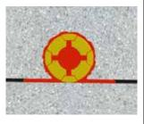
Begin injecting the SikaFuko<sup>®</sup> hose until the material flows out of the opposite end.
