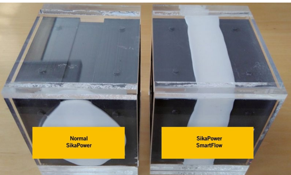
FIGURE 4 Adhesive distribution with SikaPower Standard (left) and SikaPower SmartFlow (right) (© Sika)
