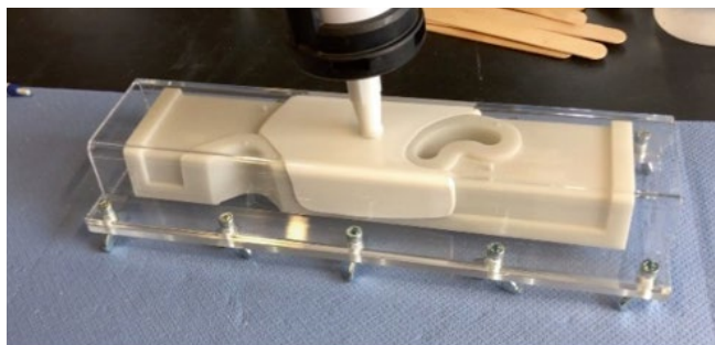
FIGURE 5 Injection into various channel widths (© Sika)
