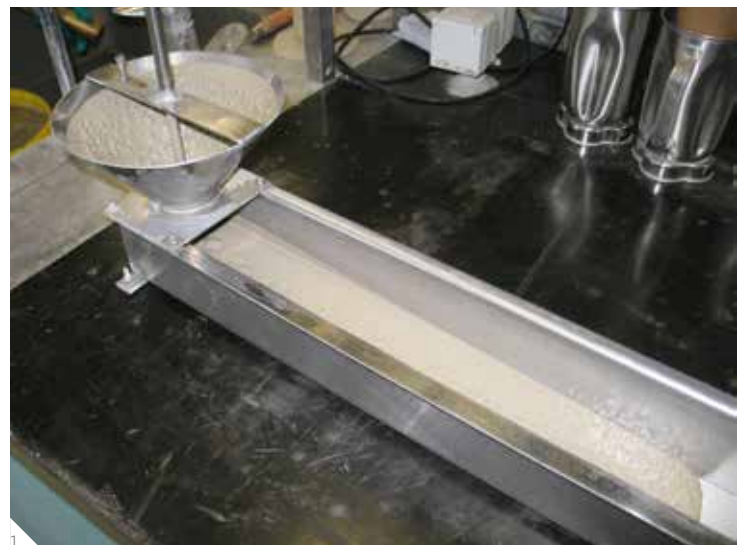
1 Flow channel for grout testing
