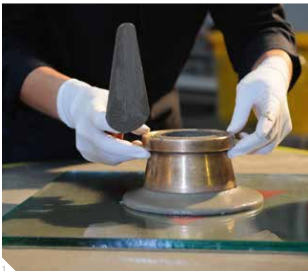
1 Flow test with Hägermann cone 2 Optimized flow properties
