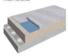
The membrane is adhered to the full surface of the substrate, giving the highest quality of aesthetic appearance. This type of application can be carried out in 2 ways:
