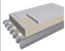
The partially adhered system is used with felt backed membranes and Sika-Trocal® C 300 adhesive, ideally suited for use on large industrial roofs. For very large roofs an adhesive application trolley cart is another practical Sika innovation.
