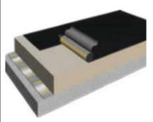
Self adhered membranes have a factory manufactured adhesive film on the back side of the membrane which is rolled out and bonded directly to the substrate when its release liner is removed.
