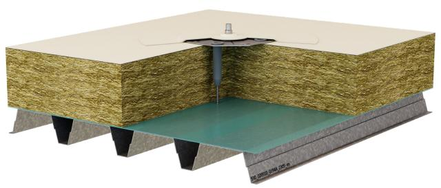
SikaRoof® Anchor Washer 140 mm fixed with Sarnafast® Fastener SBF-6.0 together with Sarnabar® Tube SBT-20. This system is used if the compression strength of the thermal insulation is slightly below 120 kPa. The maximum load per anchor needs to be reduced accordingly.
