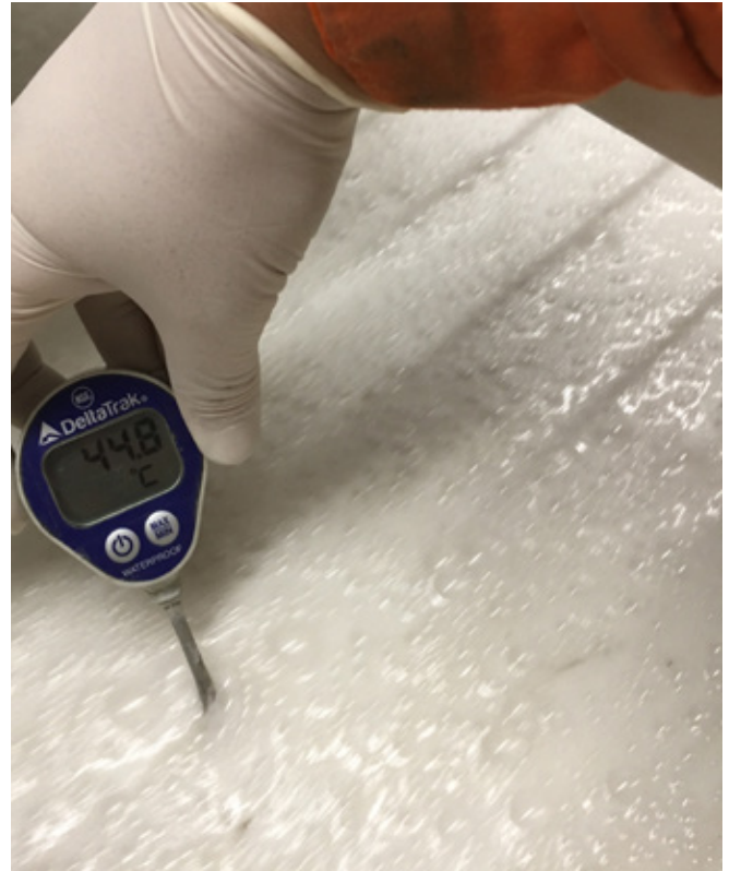
Final, mixed Sigunit L500 AF shotcrete accelerator that has been produced at the mine site blending Sigunit P-10 AF powder with water
