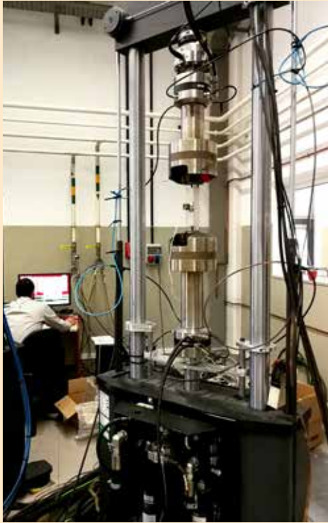
Crack bridging testing in lab.
