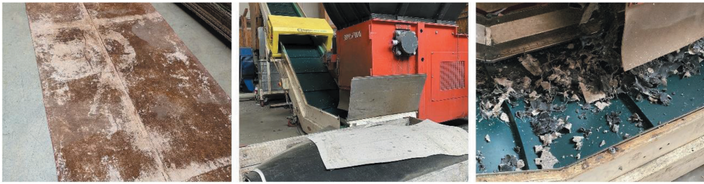
Figure 3. Different phases of the material recycling process: cleaning, shredding, and grinding.
