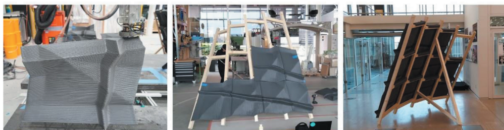
Figure 7. Final shingle, assembly, final mockup.
