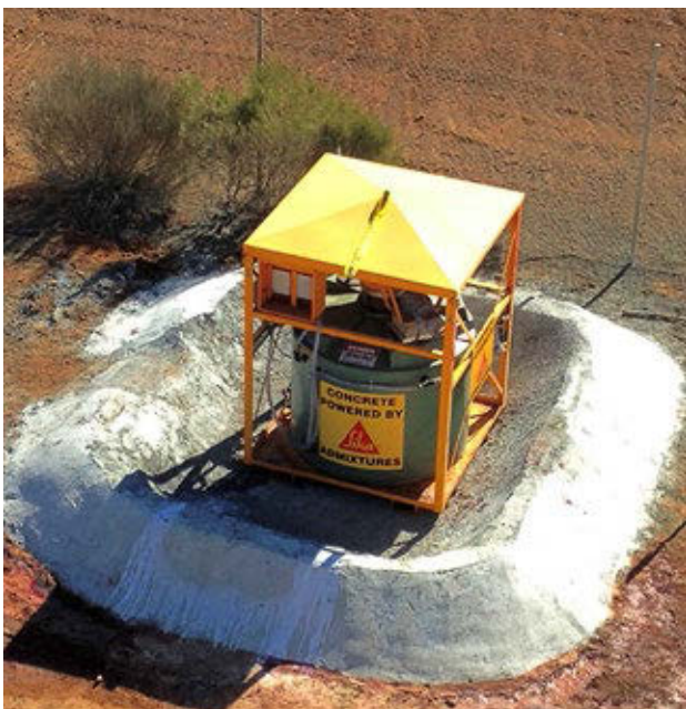
Figure 3: Simple site mixing equipment for producing liquid Sigunit® accelerator from instant Sigunit® powder
