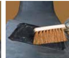
Clean the prepared surface with a soft brush or cold-air blower (use clean air)
